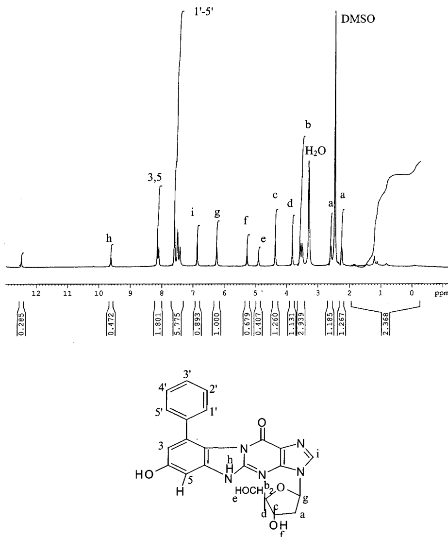
Figure 4. Spin decoupling ^1\text{H} NMR spectrum of PBQ- ^2\text{N} -dG adduct obtained from incubation of phenylbenzoquinone with 2'-deoxyguanosine (0.05 M phosphate buffer, pH 7.2) at 37 °C for 48 h. The sample was purified by preparative and analytical HPLC before determination of the spectra. The Bruker AM-600 NMR spectrometer was operated at 600 MHz and \text{Me}_2\text{SO}-d_6 was used as solvent.
